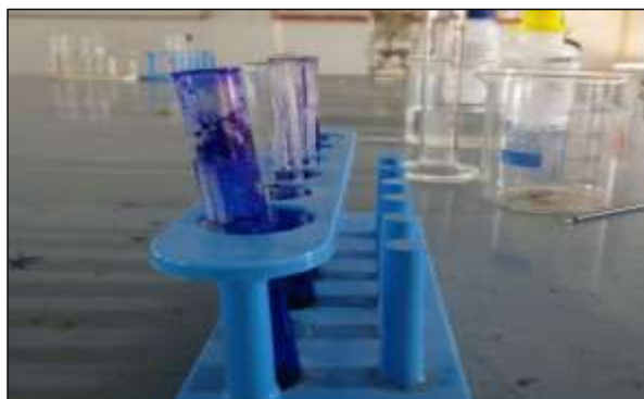
Figure 7: Blue Ink Sample collected in Test Tube by dissolving 10ml of Methanol
